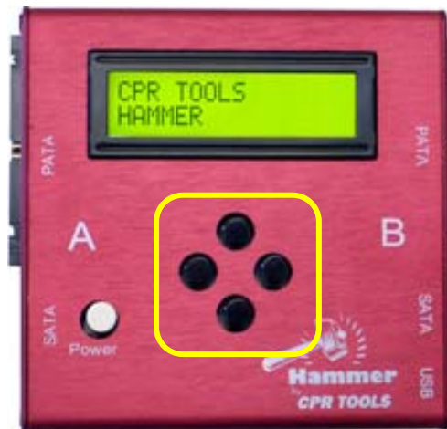
Figure 5 - Hammer™ - Navigation buttons
